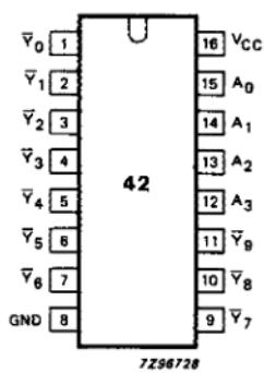
Fig.1 Pin configuration.
